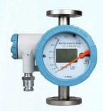
MAF 900 VARIABLE AREA intelligent metal tube flow meter is based on the floater position measurement. It has features like full metal structure, low pressure loss, big range ratio, optional transmitter with HART communication function. It is widely used in the various industries under complex and bad environment. It uses to measure the flow and controlling the process to the small flow and low velocity in all kinds of harsh conditions of medium..
